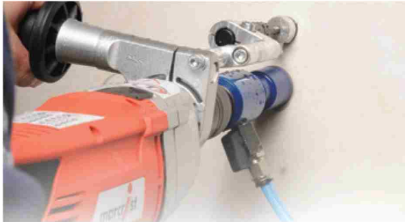
PG850: For tilers and professional users. Every hole perfect, clean and tear-free
