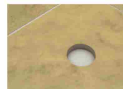
Edge drilling without breakage
