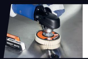
Surface finishing operations, such as satin finishing and polishing with felt flap and finishing discs.
